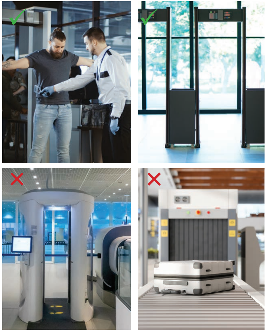
Figures 1a to d. Safe airport security screening methods. (a, top left) Handheld metal detector wand. (b, bottom left) Full-body scanner. (c, top, right) Metal detectors. (d, bottom right) Hand luggage x-ray machines.
